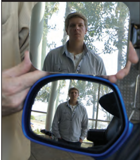
REGULAR MIRROR (ABOVE) AND CONVEX MIRROR (BELOW)
